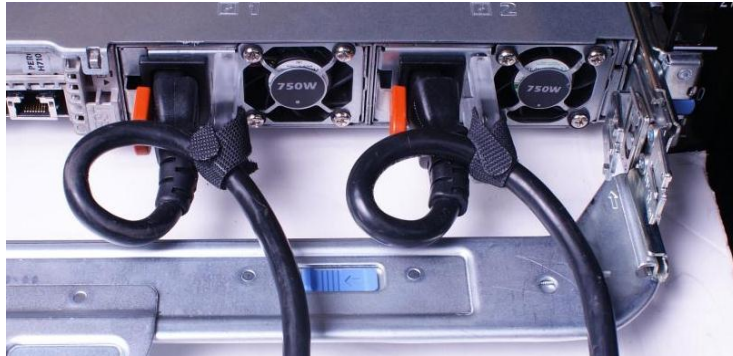
Figure 2. Routing power cables through the strain reliefs
