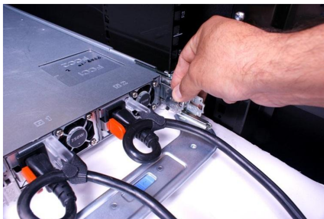
Figure 3. Attaching the inner CMA attachment bracket
